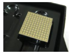
**Figure 6.** A crystal that was re-shaped and polished from an original highly irregular shape and then metallized with a solderable pixel pattern in a steering grid / guard ring arrangement. (Courtesy of Quik-Pak, a division of Delphon Industries)
