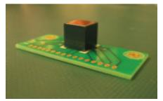
Figure 2. A detector assembly with 15mm crystal directly mounted for use in a high-energy experiment (Courtesy of Quik-Pak, a division of Delphon Industries)
