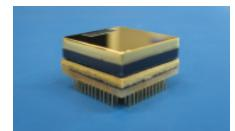
Figure 4. Detector with 20x20x10mm CZT crystal showing planar cathode and guard ring. (Courtesy of Quik-Pak, a division of Delphon Industries)
